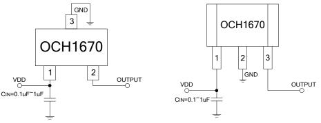
Figure 1, application circuit
