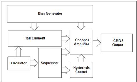
Figure 2, Block Diagram Of OCH1670
