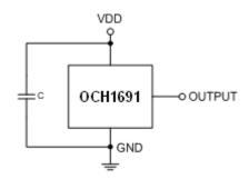
Note: C is for power stabilization and to strengthen the noise immunity, the recommended capacitance is 10nF~100nF.
