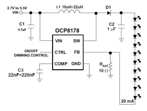
Figure 2, Typical Application Circuit of OCP8178
