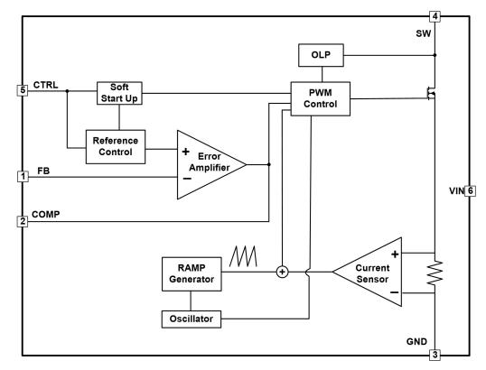
Figure 3, Block Diagram of OCP8178
