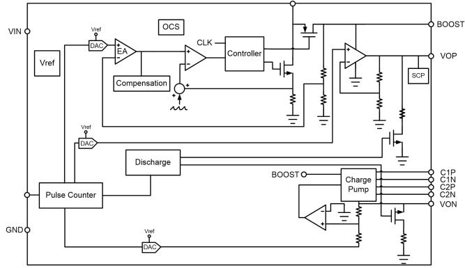
Figure 3, Block Diagram of OCP2135
