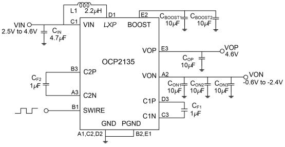
Figure 2, Typical Application Circuit of OCP2135
