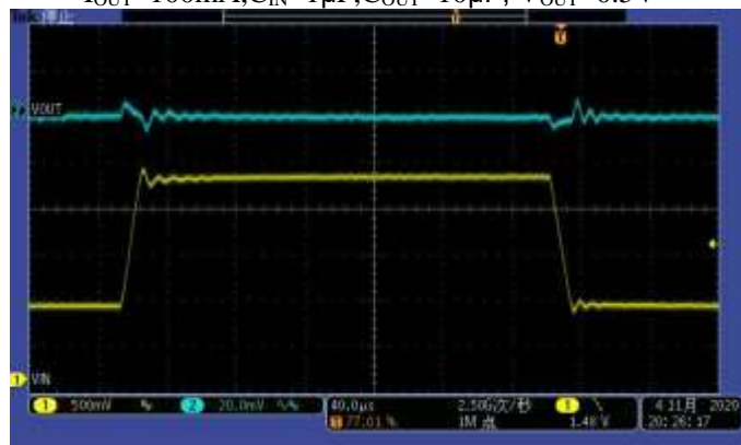
V_{IN} Line Transient Response V_{BIAS}=3V, V_{IN}=0.8-2.2V, I_{OUT}=100mA, C_{IN}=1\mu F, C_{OUT}=10\mu F, V_{OUT}=0.5V
