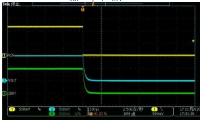
Enable Transient Response V_{BIAS}=3V, V_{IN}=1.3V, I_{OUT}=1A, C_{IN}=4.7\mu F, C_{OUT}=10\mu F, V_{OUT}=1V
