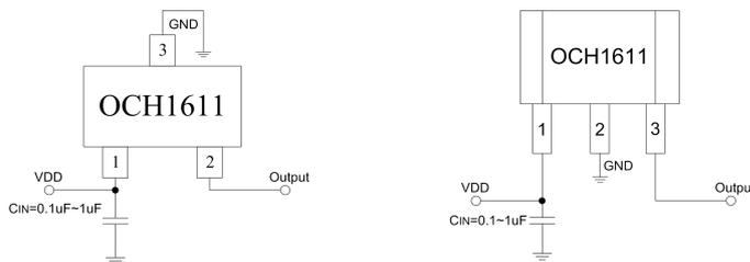
Figure 1, application circuit
