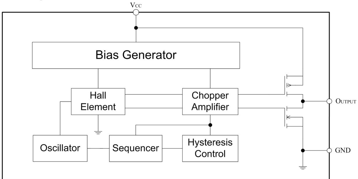
Figure 2, Block Diagram Of OCH1611
